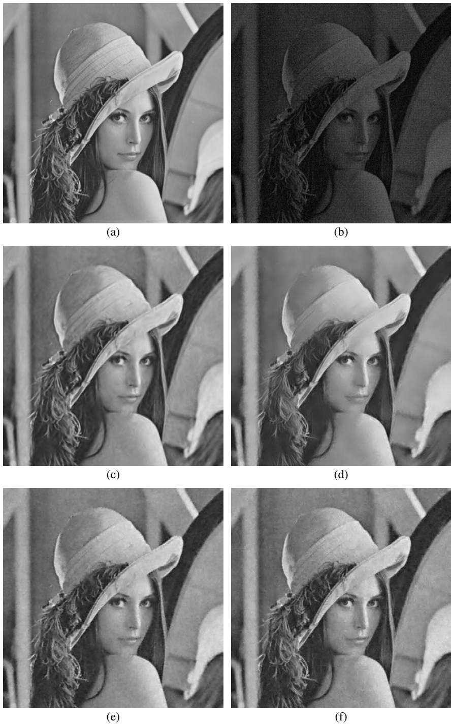
FIGURE 9.9 Reconstruction of the Lena image given a simulated noisy sensor data: (a) noise-free original color image, (b) color version of simulated noisy sensor data, (c) estimated with demosaicking method in Reference [7] and denoising method in [23], (d) estimated with the approach in Section 9.5, (e) estimated with the approach in Section 9.6, and (f) estimated with the approach in Section 9.7.
