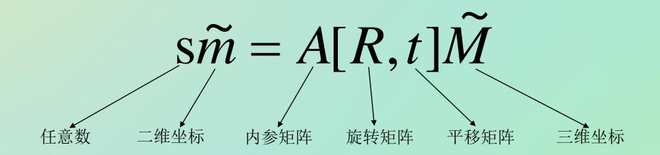
$$A = \begin{bmatrix} \alpha & \gamma & u_0 \\ 0 & \beta & v_0 \\ 0 & 0 & 1 \end{bmatrix}$$
